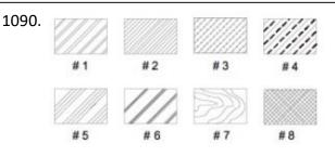
Referring to the figure, which of the following is a material section drawing for Bronze?
